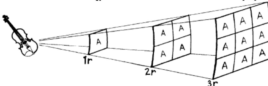
The surface area  $A$  which occupies a portion of the propagated sound wave follows the square of the distance from the sound source. The decrease in **sound intensity** (energy) follows the "**1 / r<sup>2</sup> law**" (**Inverse square law**).
